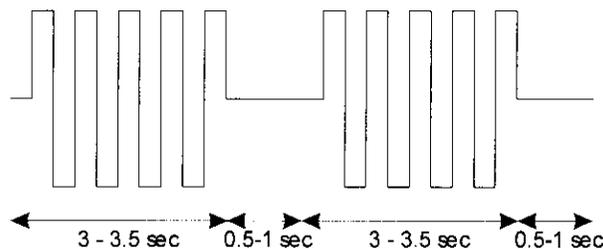
It is still the same continuous mode with a continuous train of impulses (3-3.5 sec) with a small pause (0.5-1 sec) in between.
